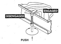
STEP FIVE — Install 4 casters D into legs of end frames A and pin with snap pins E. Set brake on each caster.
